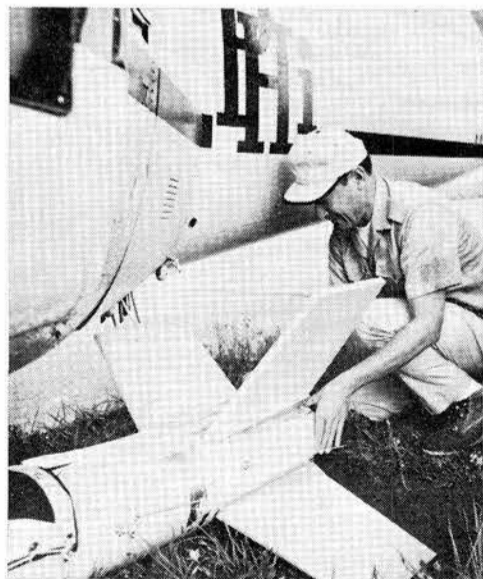
INSTRUMENTED PROJECTILE is secured to underside of helicopter by Horace Lucero (9324).
